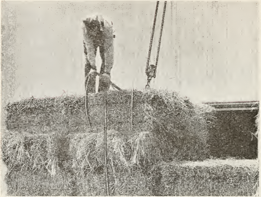
FIGURE 21.—Here, tines of the grapple fork are placed in position to lift nine bales. By this means, unloading with power forks can be done with a minimum of strenuous labor and with a small crew, especially if the hay is not stacked in the barn.
